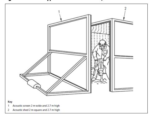
Figure A5.10.1: Typical acoustic screen/shed detail
